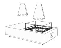
**Step 2** - Some models use two different cone heights. Place the taller cone inside the burner/pebble tray area.
