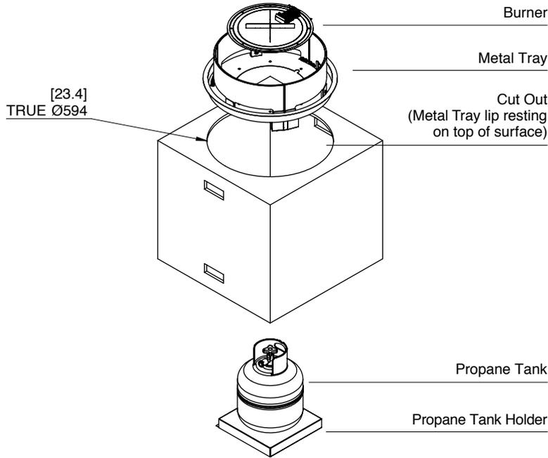
NOTE: Retention means must be provided to limit the movement of the LP gas cylinder.
